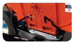
• Adjustable hopper fits virtually any door width. The sump placement below the hopper provides continuous flow rate, minimizing seed damage.
