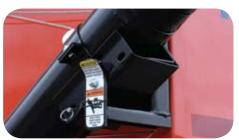
• Transport bracket with locking pin holds auger tightly to side of wagon during transport. Locking winch easily raises and lowers unit from transport position to desired working height.
