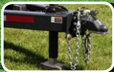
Standard heavy-duty jack, 2 5/16" ball hitch for easy hitching and transport chains.
