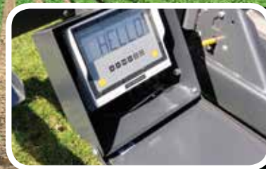
Scale for verifying seed delivered/loaded is enclosed in weather-tight box.
