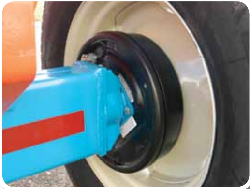
Optional 2-wheel drum-style surge brakes available on the Model 1396 provide safer road travel.
