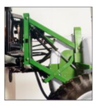
The parallel-lift system provides smooth boomheight adjustment and superior crop clearance.
