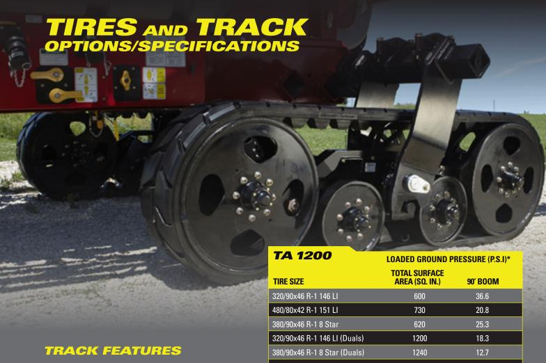
The patented Equalizer® track system provides greater flotation and offers many exclusive features.
