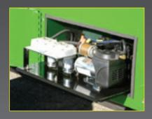
The *foam marker* uses water from the rinse tank and mixes solution at the boom for a consistent and highly visible foam. It is conveniently housed adjacent to the storage bin and comes with in-cab controls for operator convenience. Foam marker tray slides out for easy maintenance.
