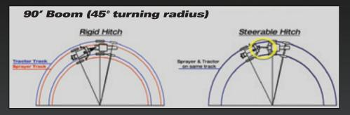
Minimize the amount of crop damage by creating just one set of tracks on the headlands with the Top Air steerable hitch option. Available with ISO, 4400 or stand-alone controllers.
