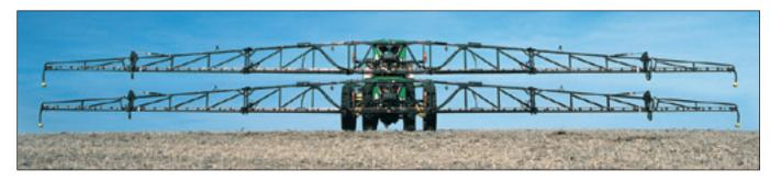
The boom's closeness to the trailer provides optimum rigidity and less stress for extended boom life. You can control the boom height on the go, from 19" to 76", meeting the most demanding spray requirements.
