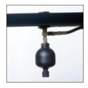
Hydraulic accumulators on lift cylinders and on wing tilt provide 16" of vertical travel independent of the trailer, for optimum leveling in extreme field conditions.
