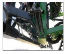
Side-mounted shock absorbers add cushioning and support to ensure level boom performance.
