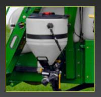
The 15-gallon chemical inductor lowers to waist level and is equipped with a large lid for easy filling. It offers high-speed chemical induction and utilizes the pressure side of the pump for better mixing of wettable powders and greater pump life. It has a spring assist for returning to storage position and features a container rinse.
