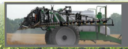
The far end of the boom, equipped with regular valves, is still spraying 2 seconds after shut-off, while the near side of the boom, equipped with FLO-BAK® valves, shuts off nearly instantaneously.
