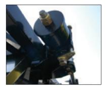
Top-mounted cushioning system provides added yaw protection.
