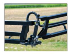
Outer wing sections feature a spring-loaded breakaway system that allows the boom wing to quickly return to spraying position should it come in contact with an obstruction.
