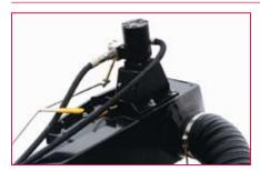
The high-efficiency orbital motor is mounted near the top of the conveyor for a cleaner operating environment, longer seal life and greater under-hopper clearance. Speed is easily adjusted from 0–500 rpm. An optional electronic on/off control is also available for easy, one-person filling and greater operator convenience.
