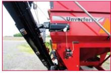
The Unverferth gravity box conveyor tucks securely to the side of the gravity box when not in use for enhanced transport safety and storage space efficiency. The unique swivel-cable design allows smooth and easy side-to-side movement. The tube-mounted friction-disc winch provides easy vertical adjustment, while the quickreleasing secondary winch permits easier transport latching.
