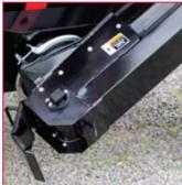
The easily accessible lower cleanout door simplifies conveyor cleanup between hybrids.
