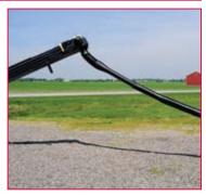
The 16'conveyor length and standard 3-stage telescopic downspout that extends from 6' to 10' stretches to a 44' reach for easily filling a 16-row planter.
