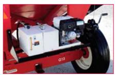
For self-contained hydraulic operation, an optional Power-Pack unit with 8 HP electric-start Honda engine is available. An optional mounting kit permits easy installation to the rear of the gravity box.
