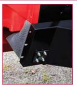
The universal mounting bracket allows for matching the Unverferth gravity box conveyor to most gravity boxes with door-angle widths ranging from 29½" to 62".
