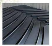
Exclusive belt design with shallow tread belt pattern for greater flotation and traction
