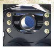
Patent-pending pivot allowing bi-directional rotation of the track for better contact with the ground on uneven terrain
