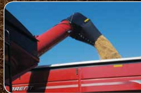
Standard 60° turret-style downspout for maximum unloading control.
