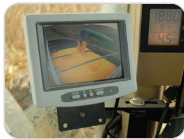
Cab-mounted monitor for side- and rear-view cameras
