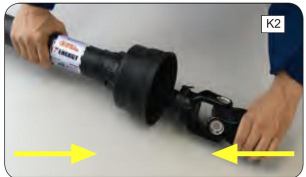
3. Slip on half-guard by aligning the holes on the cone with three bearing ring tabs and the cone inner key with the cut of the bearing ring. (FIG. K2)
