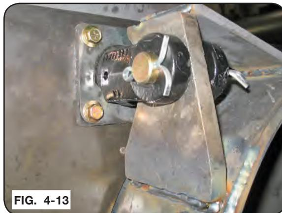
4. Remove all tools and extra hardware from the grain cart. Make sure all personnel are outside of the hopper. Then, retract the cylinder so that there is about 8" of clearance between the cylinder clevis and the lug.
