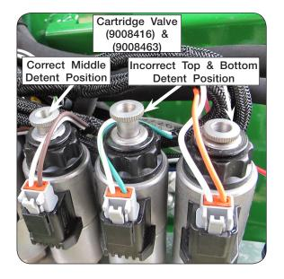
Cartridge Valve (9008416) & (9008463) Middle Detent Position
