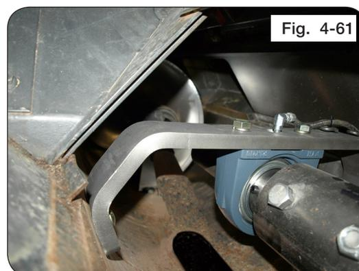
24. Extend a string tightly from front to rear to check horizontal auger alignment. Measure the string to the auger tube either in front or behind the hanger bearing. If this dimension is 1/8" greater than the measurement taken in the front and rear, shims (8GA - 286419B or 12GA - 286424B) are required on top of the center hanger bearing. Ideally the center measurement should be equal to or 1/8" lower than the measurements on the ends of the augers. (Figure 4-62)
