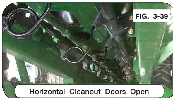
6. Remove lynch pin from rockshaft and rotate handle counter-clockwise and clockwise to check for smooth door operation.
