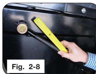
**Auger Spout Rotate Shipping Bracket Removal**
