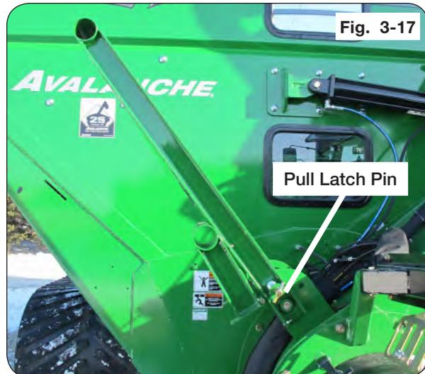
3. Fold auger down to road transport position. (FIG. 3-18)
