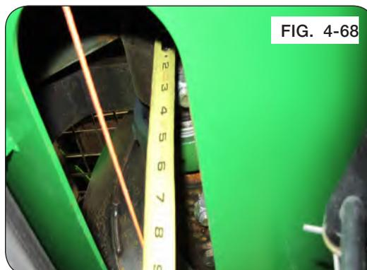
**NOTE:** The shims are 1/8" thick each. Add as needed. See "Auger System - Horizontal Auger Height Measurement" in MAINTENANCE section for more details.
