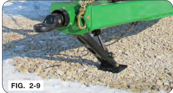
14. Remove the 1"-8UNC x 6" capscrew (9390-195) and 1"-8UNC elastic locknut (9398-026). Rotate the support stands (276748B) upwards. Reinstall the 1"-8UNC x 6" capscrew (9390-195) and 1"-8UNC elastic locknut (9398-026). Repeat process on the opposite side of the grain cart. (FIG. 2-10)
