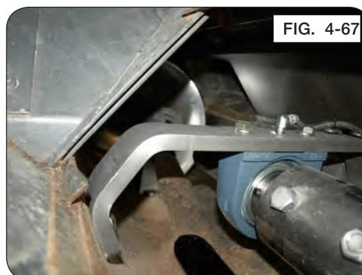
21. Extend a string tightly from front to rear to check horizontal auger alignment. Measure the string to the auger tube either in front or behind the hanger bearing. If this dimension is 1/8" greater than the measurement taken in the front and rear, shims (8GA - 286419B or 12GA - 286424B) are required on top of the center hanger bearing. Ideally the center measurement should be equal to or 1/8" lower than the measurements on the ends of the augers. (Figure 4-68)
