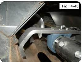
NOTE: With new flighting, the outside diameter is about 3/4" from the bottom belly pan. Always set bearing height using the 10 1/8" flighting centerline measurement. See FIG. 4-46.
