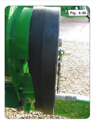
2. After tightening taper-lock bushing hardware, lay a straight edge across face of the drive and driven belt pulleys to ensure alignment between the grooves on the pulleys. (FIG. 4-31)
