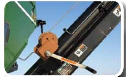
Winch system for easily moving conveyor from storage to working positions
