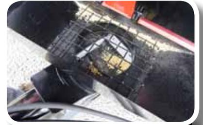
Sump-style hopper keeps conveyor full during operation
