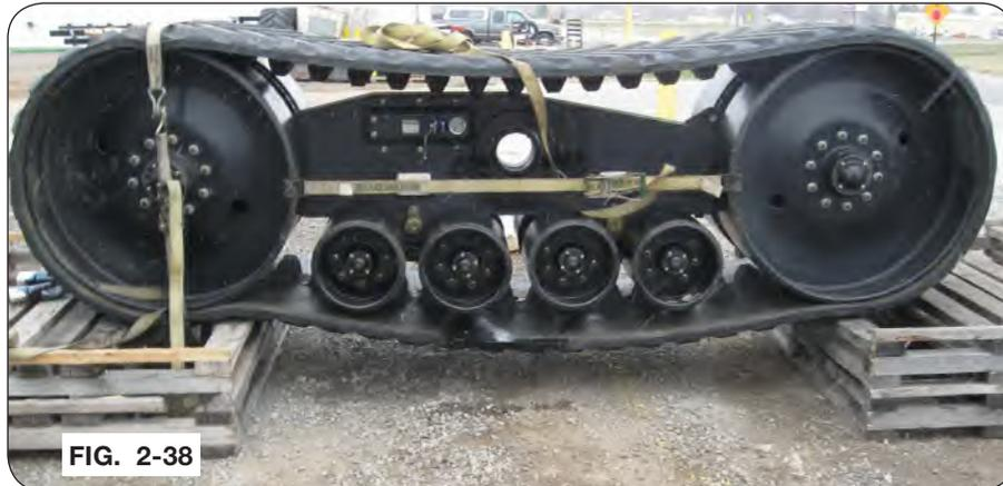
6. Hook hydraulic tensioner hose (268345) to tractor and place tractor hydraulic lever in float position. Open valve to relieve belt tension pressure and drop pressure down to zero PSI. Allow track to de-tension for 5 minutes.
