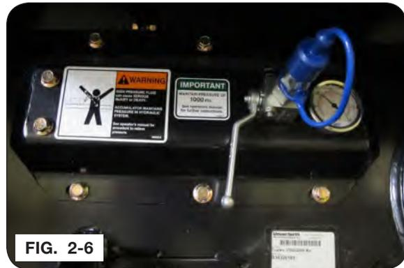
**NOTE:** If system does not hold pressure, it is possible that there is air in the lines. Follow steps 1-3 but leave the track valve open and cycle the hydraulics on the tractor from extend to float. Engage the hydraulics long enough to completely tension the track then switch it to float and allow the track to detension. Follow these steps 3 to 4 times then retension to 1000 psi and shut the track valve.
