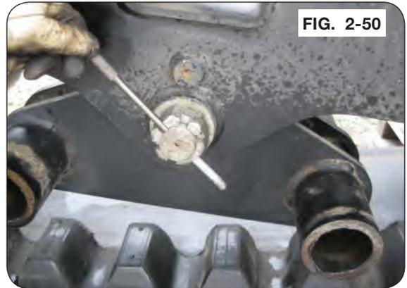
20. Reinstall the (4) spindle, hub, and bogie wheel assemblies in the same orientation as removed. Be sure to align the hole in the spindle with the spindle retaining bolt hole in the bogie pivot.
