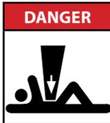
**PLACE TRACTOR IN PARK AND REMOVE KEY BEFORE DISMOUNTING TRACTOR TO ADJUST IMPLEMENT.**
