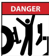
**AVOID CRUSHING.** Do not stand between tractor and implement when connecting or disconnecting implement. Injury or death can result from being trapped between the tractor and implement.
