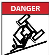
**AVOID ROLLOVER.** Do not fold or unfold implement and avoid sharp turns when on a hillside, as shift of weight could cause rollover. Operate implement at a safe distance from terrain irregularities and other obstructions that could cause rollover.
