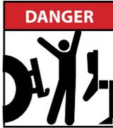
**AVOID CRUSHING.** Do not stand between tractor and implement when connecting or disconnecting implement. Injury or death can result from being trapped between the tractor and implement.
