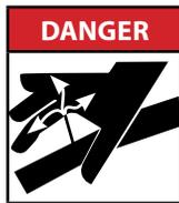
**CAUTION.** Escaping pressurized hydraulic fluid can penetrate skin, resulting in injury or death. Relieve hydraulic system pressure before connecting or disconnecting tractor. Use cardboard or wood, NOT BODY PARTS, to check for suspected hydraulic leaks. Wear protective gloves and safety glasses or goggles when working with hydraulic systems. If an accident occurs, see a doctor immediately for proper treatment.
