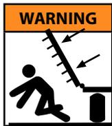
**AVOID CRUSHING.** Make sure all personnel are clear of implement at all times implement is in motion. Be aware of obstructions above, below, and around implement when in operation or transport. Injury or death can result from being struck by the implement.
