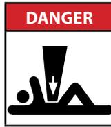
**⚠ AVOID CRUSHING.** Make sure all personnel are clear of the implement. Lower implement to the ground, place tractor in park, turn off engine, and remove key.
