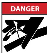
Escaping pressurized hydraulic fluid can penetrate skin, resulting in injury or death. Relieve hydraulic system pressure before connecting or disconnecting tractor. Use cardboard or wood, **NOT BODY PARTS**, to check for suspected hydraulic leaks. Wear protective gloves and safety glasses or goggles when working with hydraulic systems. If an accident occurs, see a doctor immediately for proper treatment.
