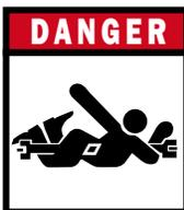
**USE BAR STANDS AND CYLINDER STOPS TO SUPPORT THE IMPLEMENT.** Store the implement on a clean, dry, and level surface. An uneven surface could cause the implement to shift or fall, resulting in injury or death, as well as implement damage. Securely support all implement components that must be raised. Store the implement away from human activity.
