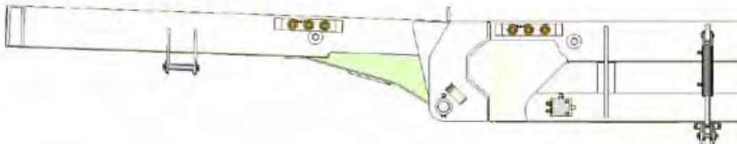
If the outer wing does not unfold far enough, remove the stop and washers in order to increase the fold angle. Repeat the alignment procedure for both outer wings.
