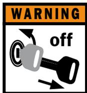
**AVOID CRUSHING.** Make sure all personnel are clear of the implement. Lower the implement to the ground, place the tractor in park, turn off the engine, and remove the key.
