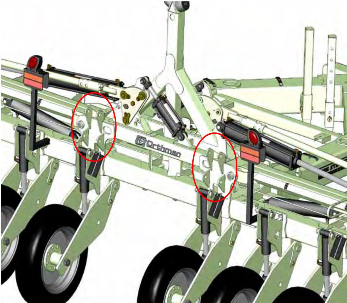
The Mount Arm package number is 399-160. The arms are designed to bridge over the lift wheels and provide depth adjustment for the Tracker 4.
