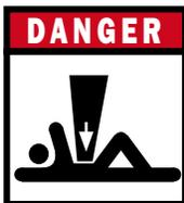
**USE BAR STANDS AND CYLINDER STOPS TO SUPPORT THE IMPLEMENT.** Store the implement on a clean, dry, and level surface. An uneven surface could cause the implement to shift or fall, resulting in injury or death, as well as implement damage. Securely support all implement components that must be raised. Store the implement away from human activity.
