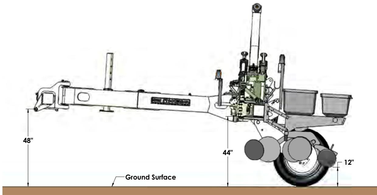
Once hydraulic tips are connected to the tractor to operator preferences, lift the tractor hitch and lift wheels. The dimensions illustrated are approximate. Be sure your implement reflects similar dimensions in the fully-raised position.
