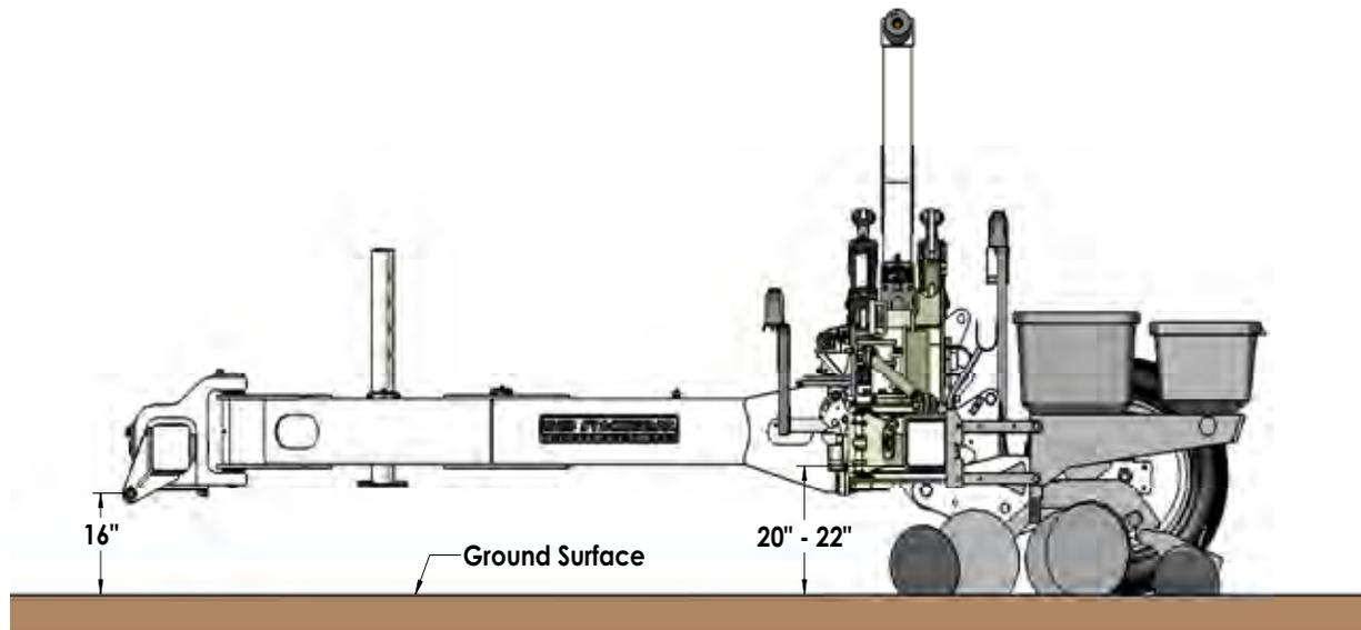
A 1925 Stacker Bar operating on level ground at 20 inches above the planting surface is shown. For this setup the lift cylinders are fully retracted with no stops. For the 22 inch operating height, a 1 inch stop is required on each lift wheel. If you are planting on beds or ridges, more stops are necessary in order to achieve the correct operating height.
