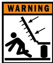
**AVOID CRUSHING.** Make sure all personnel are clear of the implement at all times that the implement is in motion. Be aware of obstructions above, below, and around the implement when in operation or transport. Injury or death can result from being struck by the implement.
