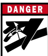
**AVOID CRUSHING.** Do not stand between the tractor and implement when connecting or disconnecting the implement. Injury or death can result from being trapped between the tractor and implement.
