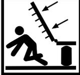
**AVOID CRUSHING.** Make sure all personnel are clear of the implement at all times that the implement is in motion. Be aware of obstructions above, below, and around the implement when in operation or transport. Injury or death can result from being struck by the implement.
