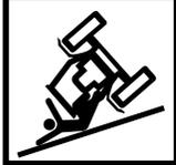
**AVOID ROLLOVER.** Do not fold or unfold the implement and avoid sharp turns when on a hillside, as shift of weight could cause rollover. Operate the implement at a safe distance from terrain irregularities and other obstructions that could cause rollover.
