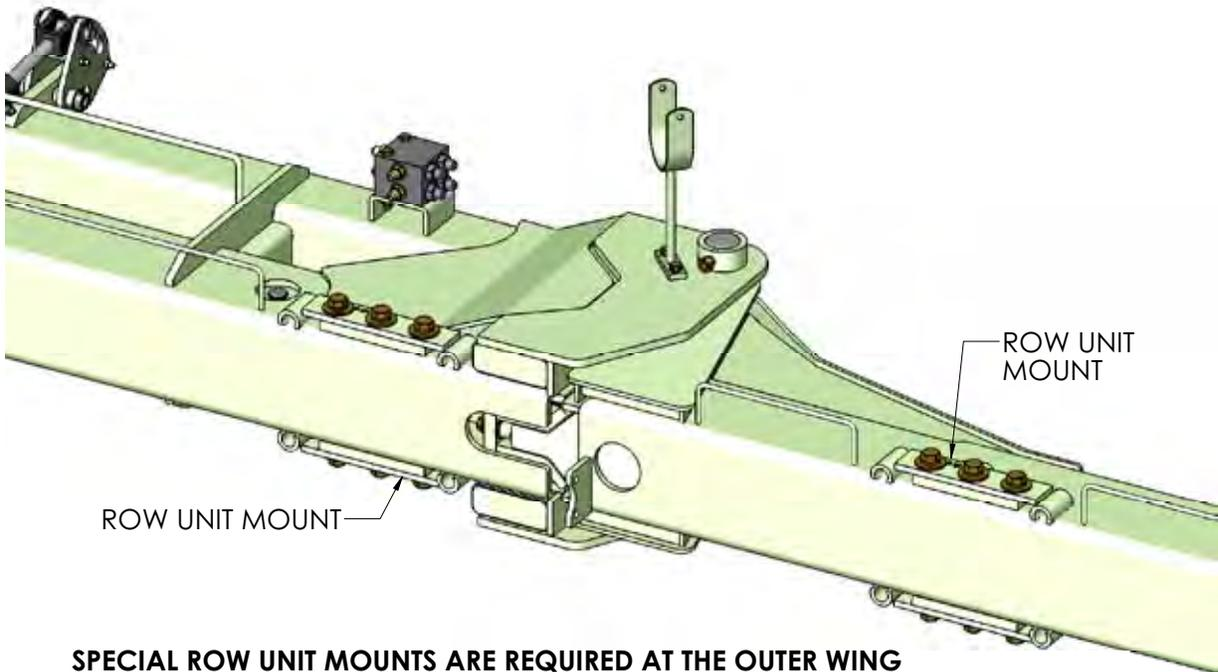
**SPECIAL ROW UNIT MOUNTS ARE REQUIRED AT THE OUTER WING HINGE ON ALL BARS AND THE CENTER SECTION ON 20-24 ROW BARS**
