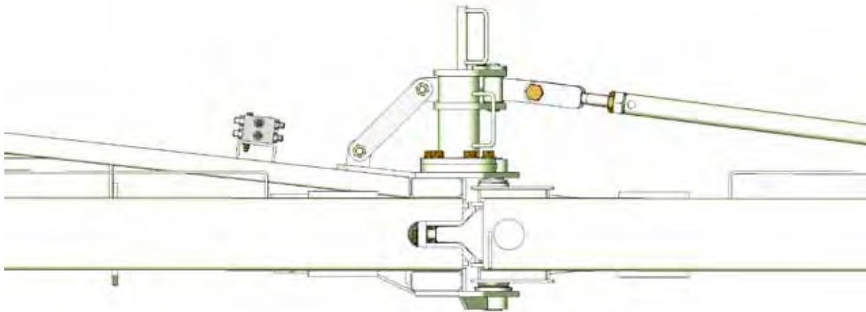
The adjustable stop is comprised of a tapped stop and a series of spacer washers.
