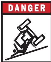
**AVOID ROLLOVER.** Do not fold or unfold implement and avoid sharp turns when on a hillside, as shift of weight could cause rollover. Operate implement at a safe distance from terrain irregularities and other obstructions that could cause rollover.
