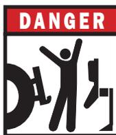
**AVOID CRUSHING.** Do not stand between the tractor and implement when connecting or disconnecting implement. Injury or death can result from being trapped between the tractor and implement.
