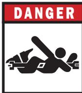
**AVOID ENTANGLEMENT.** Never lubricate or service implement in motion. Keep away from power driven parts when in motion. Disengage power sources prior to maintaining implement. Injury or death can result from contact with power driven parts when in motion.
