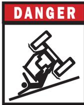
**CAUTION!** Stacking one wing at a time causes center of gravity to shift resulting in rocking and unbalanced equipment. Use extreme caution when moving unbalanced equipment, the tractor and implement are more likely to tip.
