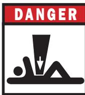
**USE BAR STANDS AND CYLINDER STOPS TO SUPPORT THE IMPLEMENT.** Store implement on a clean, dry, and level surface. An uneven surface could cause implement to shift or fall, resulting in injury or death, as well as implement damage. Securely support all implement components that must be raised. Store implement away from human activity.
