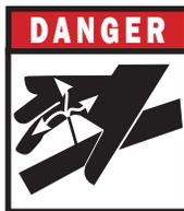
Escaping pressurized hydraulic fluid can penetrate skin, resulting in injury or death. Relieve hydraulic system pressure before connecting or disconnecting tractor. Use cardboard or wood, **NOT BODY PARTS**, to check for suspected hydraulic leaks. Wear protective gloves and safety glasses or goggles when working with hydraulic systems. If an accident occurs, see a doctor immediately for proper treatment.
