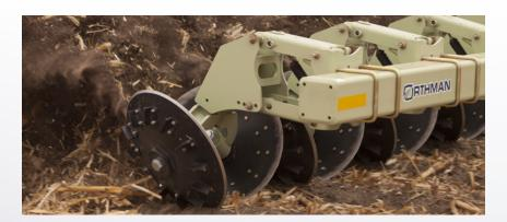
The Orthman Stalk PULLr's unique design provides dual overlapping 24" discs with drive lugs to help propel them through the field. The angle and depth adjustability allows you to determine the amount of tillage that occurs in the row.
