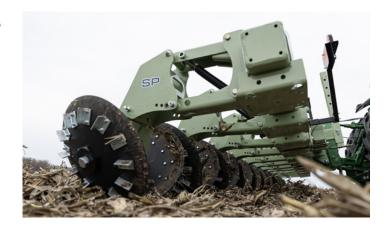
Discs feature replaceable cleats to propel them through the field at higher speeds for plug-free operation.
