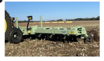
The Orthman time-tested row units feature parallel linkage for independently following the ground contour and are constructed with self-lubricating, greaseless composite bushings to eliminate daily maintenance for covering more acres per day. Downpressure is easily adjusted to match soil type and desired field finish.
