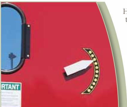
Hydraulic flow control allows the operator to feather the flow of grain from fully open, for the fastest unloading, to a slower flow for topping off trucks with ease. Standard viewing windows allow convenient checking of loads.
