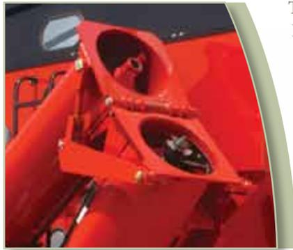
The 18" unloading auger on the 1048 unloads over 8 bushels per second, while the 22" unloading auger on the 1348 unloads over 12 bushels per second! The combination of gearbox-driven unloading auger with belt-driven in-line auger requires fewer moving parts and less starting torque than conventional double-auger carts.
