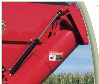
The unloading auger features a self-locking system, ensuring no grain leakage.
