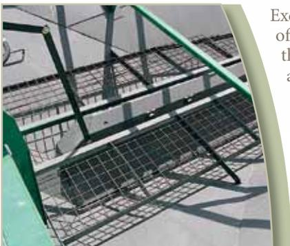
Exclusive in-line auger design offers a one-piece floor auger that force-feeds the vertical auger for lightning fast unloading times without the extra moving parts of a traditional double-auger cart.
