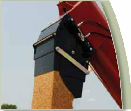
The hydraulic spout discharges the grain either straight down at a 90° angle or outward at a 128° angle for easy unloading into the center of the trucks.
