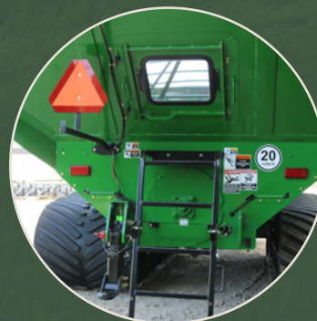
Rear tank access door
