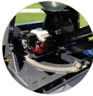
Seed Chariot model 1020 bulk box carrier is powered by a 5.5 hp/160 cc industrial-grade gas engine with electric start
