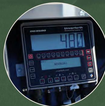
Scale for verifying seed delivered/loaded is enclosed in weathertight box
