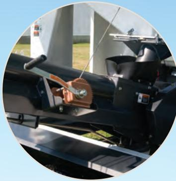
Winch-operated vertical height adjustment allows for easy filling of different planter types
