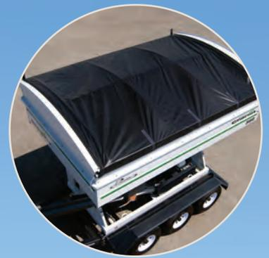
Standard 18-ounce Weatherguard roll-over tarp protects contents from weather and stays tightly locked, even at highway speeds
