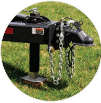
Heavy-duty jack, 2 5/16" ball hitch for easy hitching and transport chains
