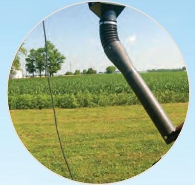
The 18' steel tube with 5' telescoping downspout can reach up to 30' and the 21' conveyor up to 36'
