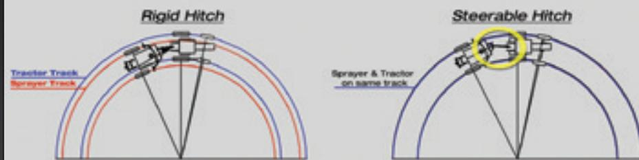
Minimize the amount of crop damage by creating just one set of tracks on the headlands with the Top Air steerable hitch option. Available with ISO, 4400 or stand-alone controllers.
