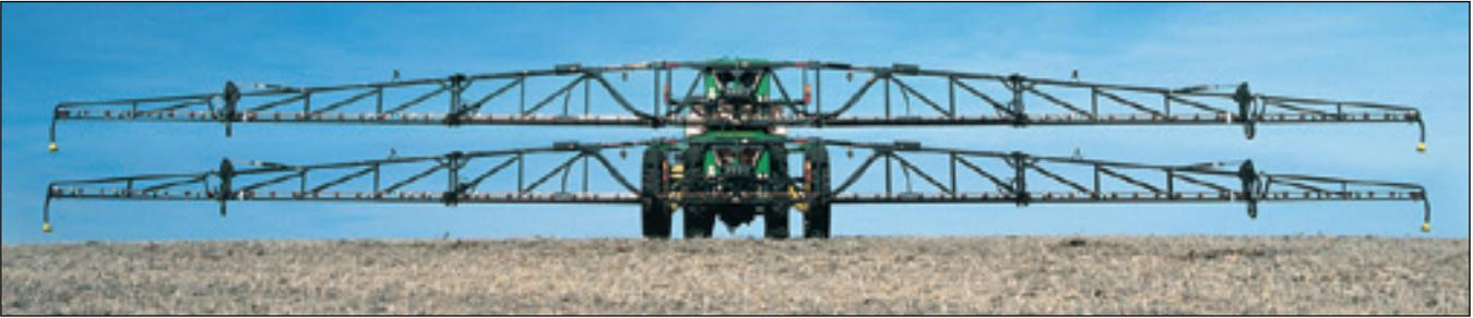
The boom's closeness to the trailer provides optimum rigidity and less stress for extended boom life. You can control the boom height on the go, from 19" to 76", meeting the most demanding spray requirements.
