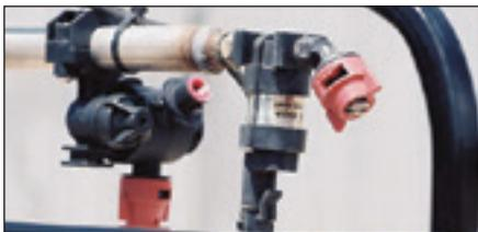
The fence-row nozzle kit comes with an angled tip for each boom end and in-cab controls for easily spraying end rows.
