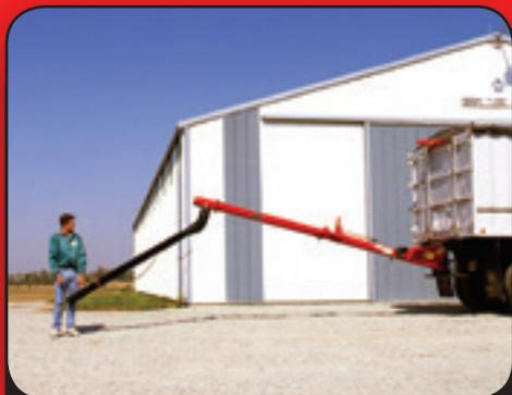
Extendible downspout from 9' to 14'9" and a 360° rotating elbow for a full 25' reach
