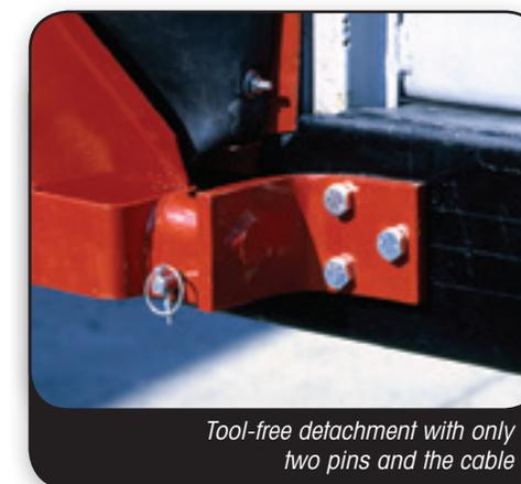
Tool-free detachment with only two pins and the cable
