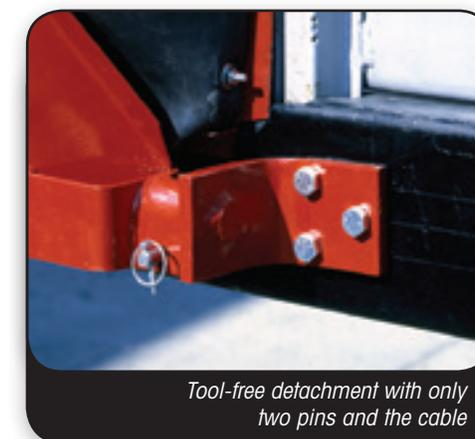
Tool-free detachment with only two pins and the cable
