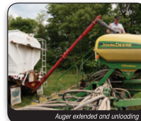
Auger extended and unloading
