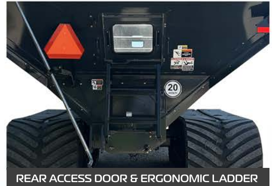
REAR ACCESS DOOR & ERGONOMIC LADDER
