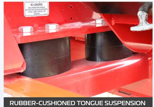
RUBBER-CUSHIONED TONGUE SUSPENSION
