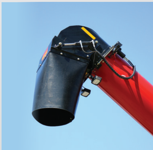
Four-way downspout with inward/outward and side-to-side maneuverability
