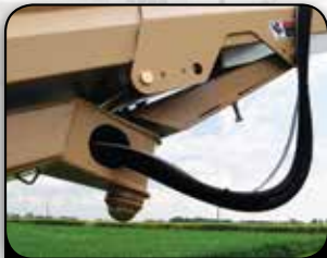
Adjustable spring-lift assist for easier conveyor movement
