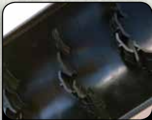
Cupped rows of offset cleats gently moves seed at up to 25 bushels per minute
