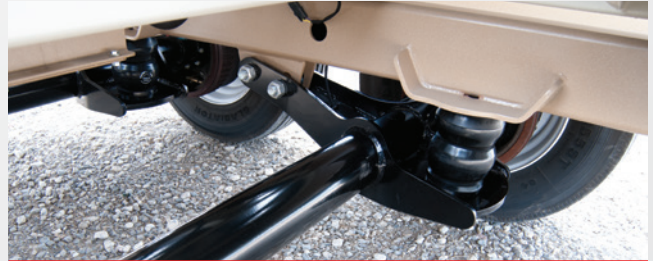
Rubber-cushioned suspension on 4955DXL, 4955XL and 3955XL
