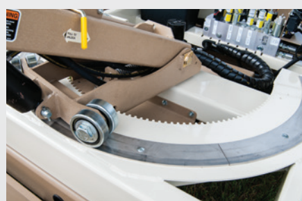
Turntable features 3/4" increments
