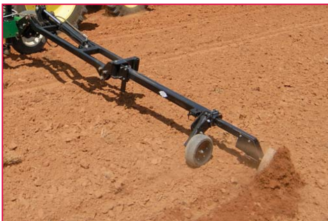
Optional shear-bolt protected row markers with notched blades leave a highly visible mark. An optional gauge wheel package for row markers on 6- and 8-row models ensures constant depth in soft soil conditions.
